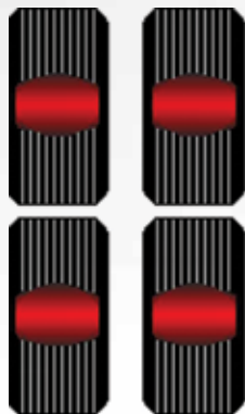
After getting each tire contact patch equally loaded across its width, the goal is to have all four tires equally loaded as much of the time as possible.
