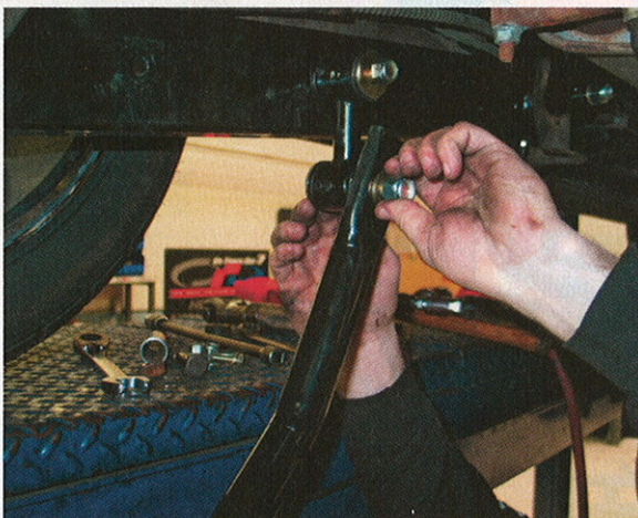
The Elky's factory lower trailing arms show attempts at reinforcement, but are still weak, especially when compared to the fully boxed Hotchkis replacement. With stronger arms and polyurethane bushings in place, wheelhop is reduced and stability improved.
