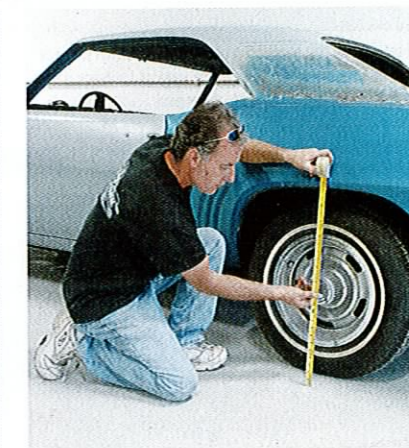
Competition Specialties team member Paul Thetonia took a second to measure the car's rear height from the ground to the top of the rear wheel opening before the Hotchkis suspension was installed. It came in at 26 3/8 inches.
