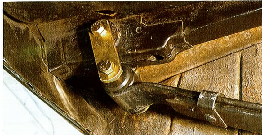
Using more of the provided lube, the rear bushings are installed into the new leaf spring, and the rear of the leaf is finally mounted securely into place.
