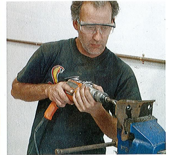
The preparation for installation of the new Hotchkis rear suspension components requires some minor modification to both the upper and lower spring perches to accommodate the beefier U-bolts supplied in the kit. Here Paul drills the lower spring perch with a 5/8-inch drill bit.
