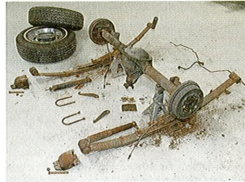
Completely blown apart with decades of well-earned rust still on the ground, the only thing to be reused will be the rearend—once it's taken apart, checked, and freshened up.
