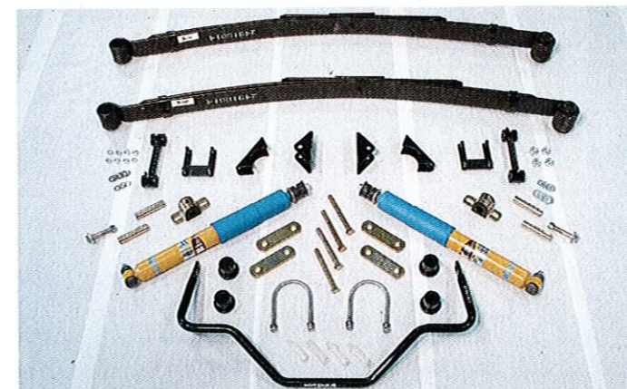
For killer handling, it doesn't get any better than installing a full Hotchkis rear suspension. To make sure the rear of the '69 will keep planted to the ground, the team from Competition Specialties ordered up a complete front and rear TVS small-block suspension system along with a set of HPS 1000 shocks. You can also just order up the rear Sport Leaf Spring Package complemented by the Sport Sway Bar Package and a pair of HPS 1000 rear shocks if you choose. Hotchkis kits are available in any combination, and they always include complete mounting hardware and instructions.
