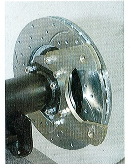
Next, slide the new rotor onto the axle hub.
