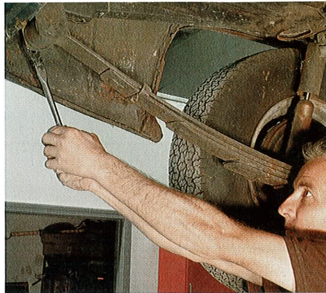
After using some rust penetrating oil and a ratchet, Paul was able to loosen the spring perch bolts without a problem. Note that since a lift is being used, all hardware is only being loosened at this time for final removal once the car is lowered to the ground.
