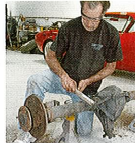
Gee, poor Paul always gets stuck with the clean up! Here he uses a wire brush to remove any rust on the rearend to be followed by degreaser, 80-grit sandpaper and scuff pads in getting it ready for a fresh new look.
