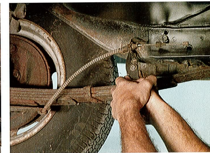
Paul first removed the front section of the emergency brake cable line and then followed up with removal of the rear section. The new installation kit from Master Power includes a complete emergency brake cable package.
