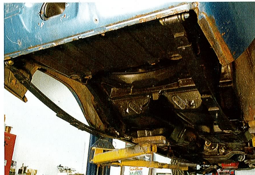
With the freshly repainted and detailed undercarriage of the '69 looking fine, the new Hotchkis springs are ready to accept the rearend to complete the installation.
