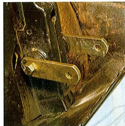
Once the rear spring perch is cleaned thoroughly, it's lubed with the provided product from the kit, and the new bushings and heavy-duty rear shackles are installed.
