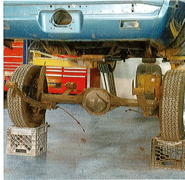
With the car lowered and the rear wheels on a pair of milk crates (you could also use jack stands), Paul removed all of the loosened hardware and the car was lifted up slowly while the entire rear suspension was removed. Let the fun begin!
