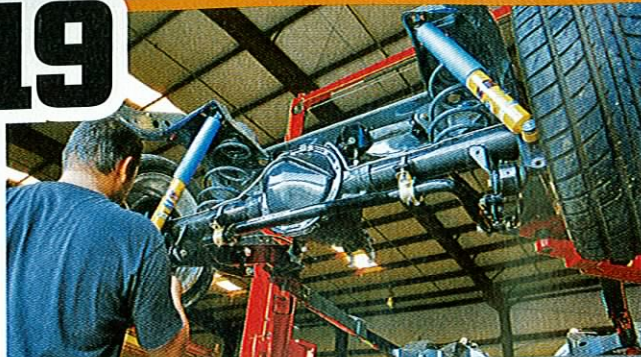
The tubular rear sway bar offers two adjustment options, 75 and 100 percent stiffer than stock, so you can fine tune rear roll stiffness for optimum traction. All the hardware, bushings, etc. are in the TVS kit for the rear sway bar.
