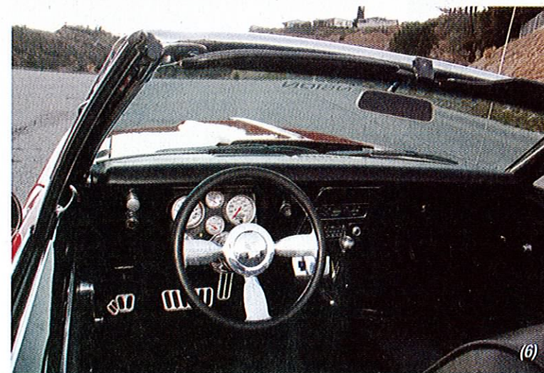
(6) Upgrades to the interior include a new Painless 18-circuit wiring harness, AutoMeter gauges, a Lokar billet shifter and a slick center console pirated from a 1998 Camaro.
