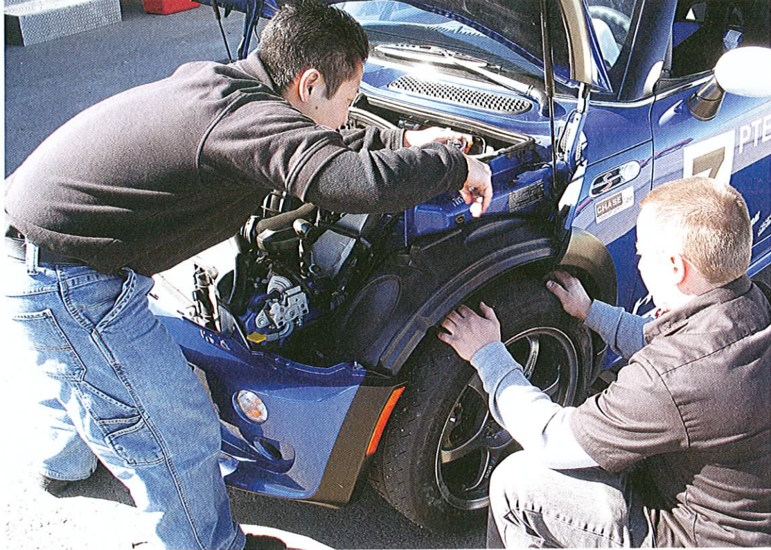
Aaron Ogawa and Corey Bedortha (kneeling) adjust the camber on our MINI Cooper S test car. This particular MINI runs Bilstein PSS9 coil-overs, Hotchkis anti-roll bars and a set of their adjustable camber plates. John Hotchkis (below) also helped with the test, taking copious notes throughout the day on how each alignment setting impacted tire temperatures and lap times.
