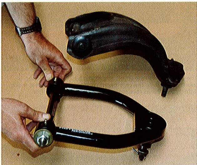
Note how the factory upper A-arm has to curve downward due to the shorter spindle, while the Hotchkis A-arm is much flatter in-configuration. This setup helps to maintain negative camber and thus better tire grip throughout the suspension travel.
