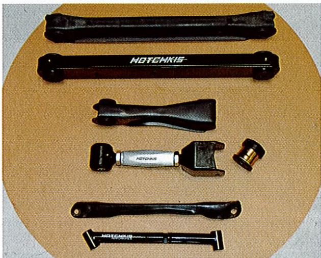
From top to bottom, factory versus Hotchkis rear suspension arms and braces. The higher quality of construction is clearly obvious, as is the adjustability.
