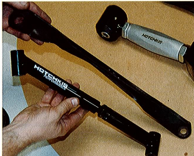
Note the difference in size, quality and adjustability of the brace for the trailing arm mount.
