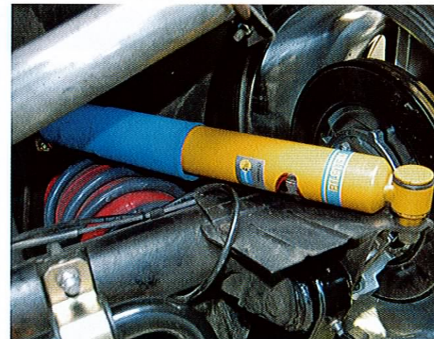
Custom-calibrated Bilstein shocks and 1-inch-lower, precision-wound coil springs provide a more stable ride and a more aggressive stance. The airbags (red) are not included.
